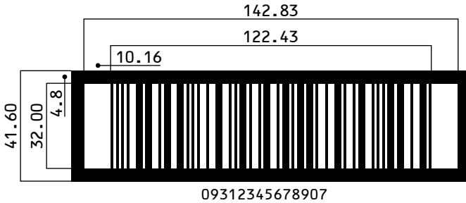
Example of a 100% ITF-14 Bar Code Symbol (Diagram is not to scale)
